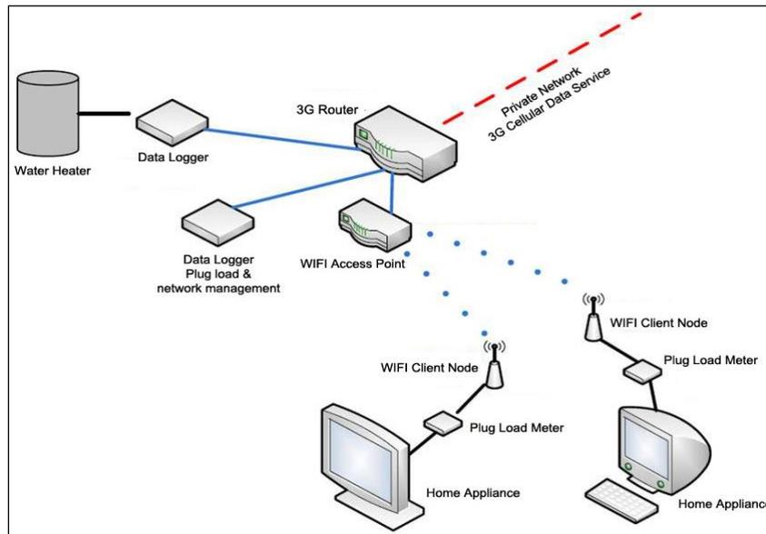
The 3G routers connect via a private cellular data network to redundant VPN routers at Ecotope. Traffic is routed through a firewall before reaching Ecotope's servers. Because the network is a cellular data network and not a phone network, connections are always live; this factor allows active monitoring of equipment, which helps ensure data quality. Finally, as mentioned above, the network is private, with no access to the public Internet.
