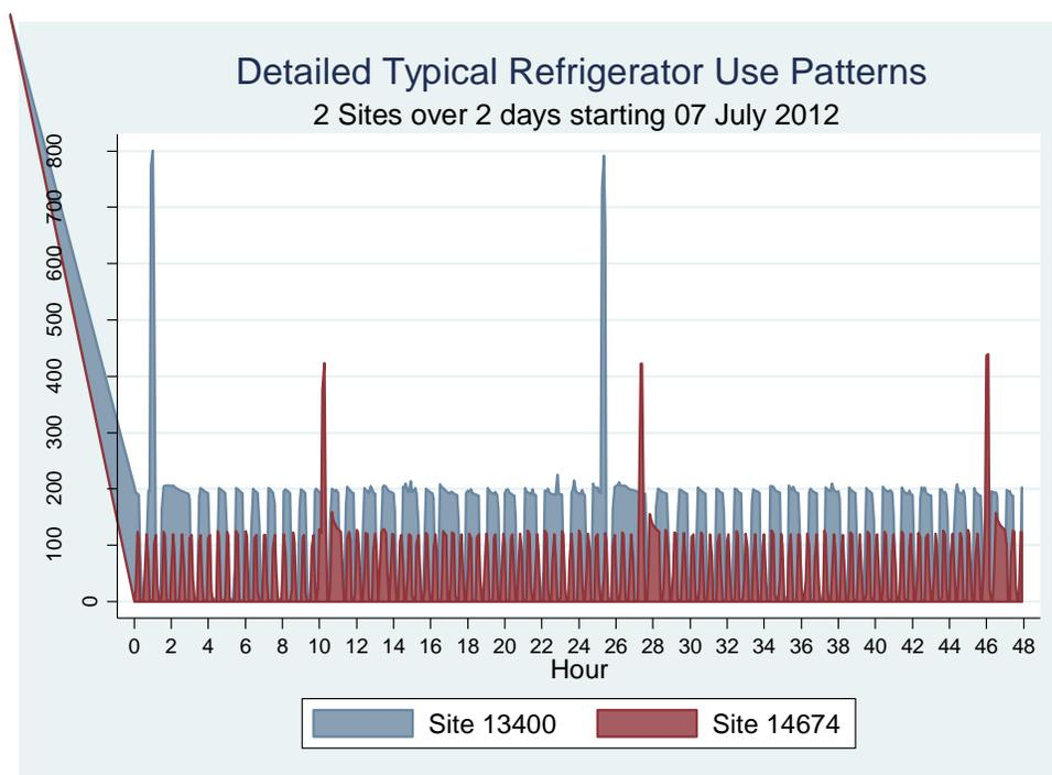
Monthly use also increases during summer months. Figure 34 shows the energy use for primary refrigerators, which are all inside the conditioned space. Usage in August averages about 1.7 kWh/day versus about 1.2 kWh/day in January. Many houses have mechanical cooling, but interior temperatures are overall higher in summer. Refrigerators in garages or basements show a different annual profile because those spaces are subject to larger temperature swings (see Appendix 8 for load shape).
