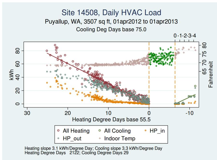
HP\_in: Heat pump indoor unit (including electric resistance)
