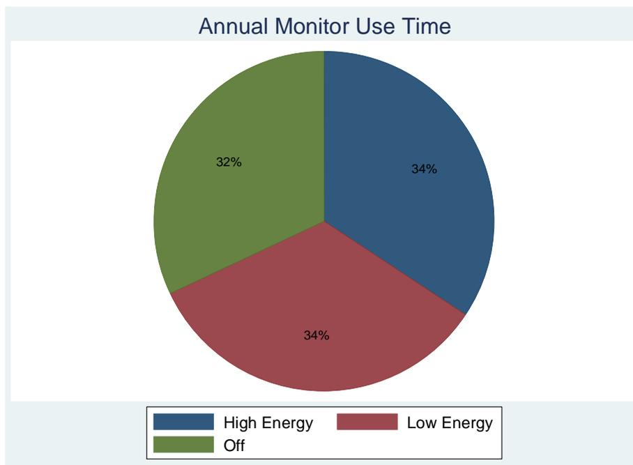
Monitors in this study used an average of 47 watts in high power mode and 2 watts in low power mode. Not only are monitors more aggressive than CPUs about powering down, but also low power mode is lower than CPUs.
