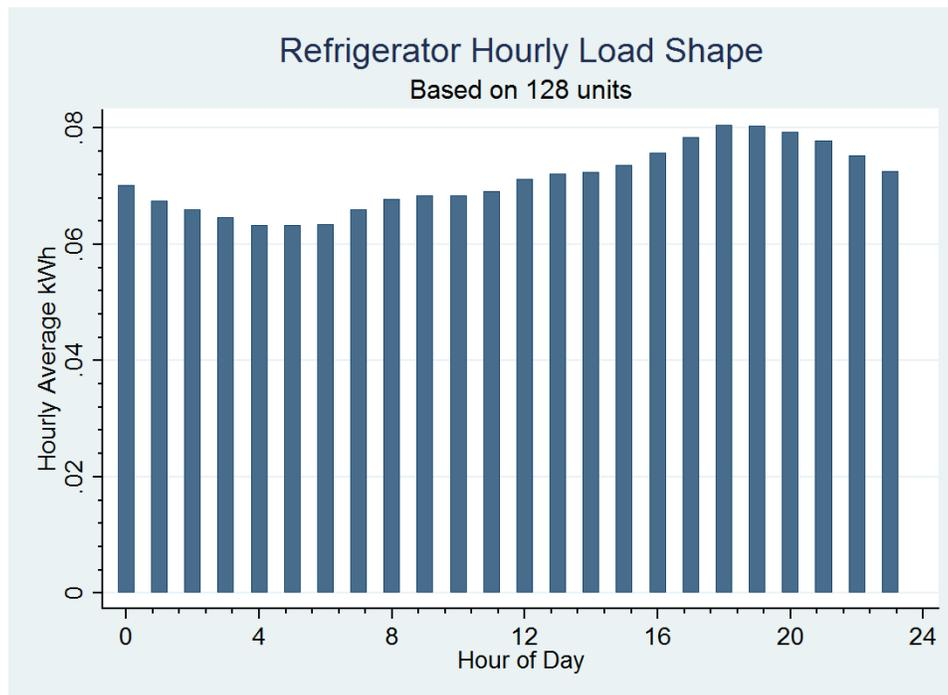
Figure 32 compares the observed hourly load shapes in the current study to the ELCAP study from 25 years ago (Pratt et al., 1990). Notably, the magnitude of refrigerator energy use is 40% today of what it was two decades ago. More subtly, the shape of the energy use has not substantially changed. The relative height between the peak and valley is still about 25% of the peak power draw although total daily use is less.
