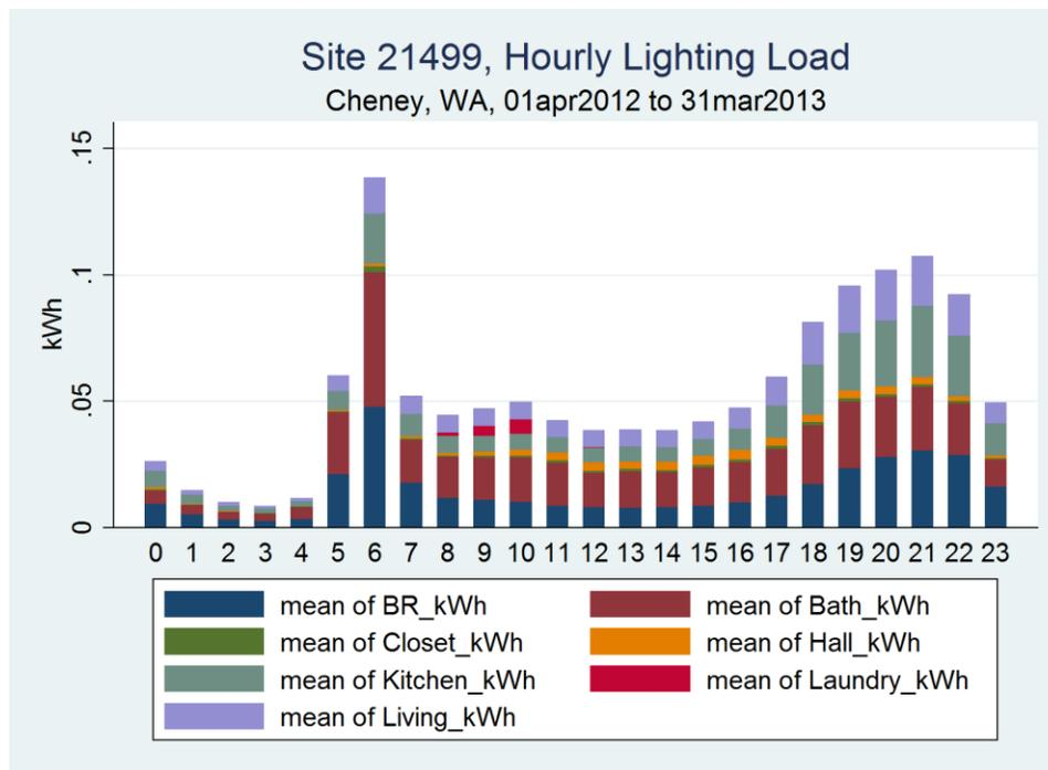
The overall lighting load shape is based on the aggregate on-time from the metered sample. It is important to note that the energy associated with this load shape is extremely mutable. The region's residential lighting has undergone a substantial change in the last decade. This trend can be expected to continue in the next decade with the advent of higher lighting standards and with new technologies, such as LEDs, that promise to further reduce the connected lighting load.
